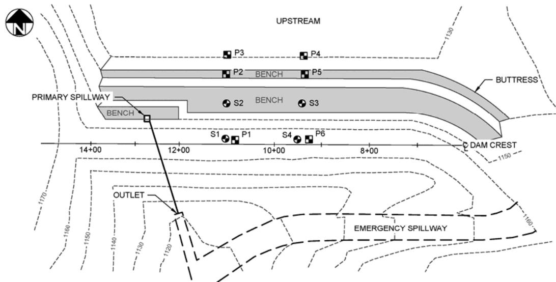
**Figure 4. Site plan after remediation**
