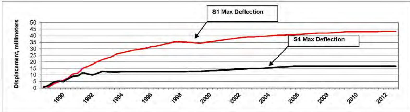
Figure 8b. Inclinometer measurements after remedial construction
